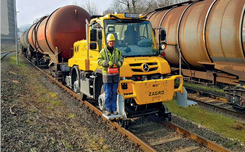
Unimog U 423 Funkrangierer, Lauffräder Ø 400 mm Unimog U 423 with radio remote control, rail wheels Ø 400 mm
