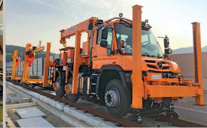
Unimog U 423 Arbeitsfahrzeug, Gelenkrollen Ø 136 mm Unimog U 423 working vehicle, rail rollers Ø 136 mm
